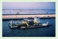
The vessel is suitable for discharging dredged soil, lifting mud, and/or applying the in-pipe-mixing solidification treatment method, in coastal constructions.
